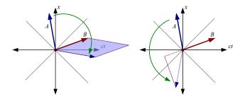
FIG. 1. Two space-time dot product visualizations which use reflections in the (ct, x) plane.
